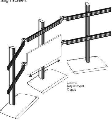
ii. Hook on the remaining flat screens and align screens accordingly.
