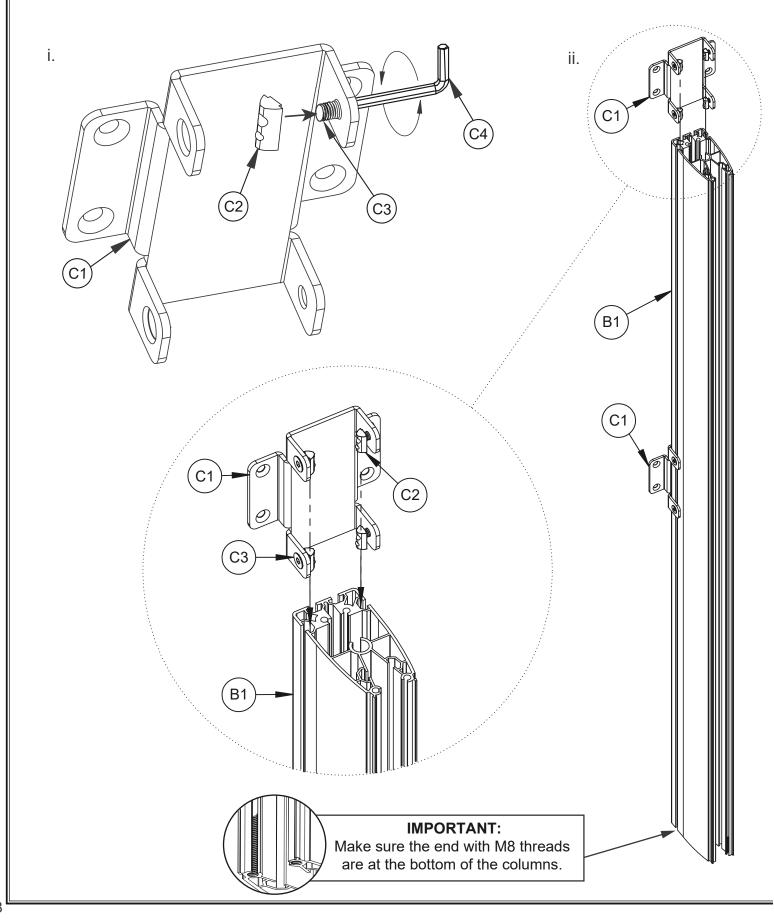
iii. Use item F1 to set the distance between items C1 on item B1 according to the screen size. Once set, tighten item C3 with item C4. 1026 × 580 **ADJUSTMENT** KNOB Leave at least a 5mm gap at top of column for item B2 0
