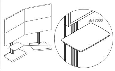
Use a *BT8390-SA* shelf adaptor to mount shelves directly under or over the horizontal mounting rails.
