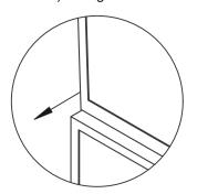
Use **Lateral Adjustment** to align sides of screens
