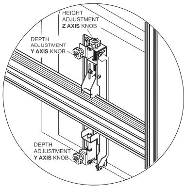
Use **Depth Adjustment** (Y axis knobs) to align front of screens
