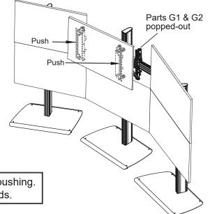
**IMPORTANT:** Be careful not to damage the screen when pushing. Keep hold of the screen as it moves outwards.
